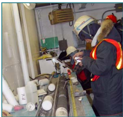
Cores recovered from the Mallik drilling operation were quickly preserved in liquid nitrogen to preserve them for later analysis of gas content, porosity, thermal conductivity, and other characteristics (USGS).
