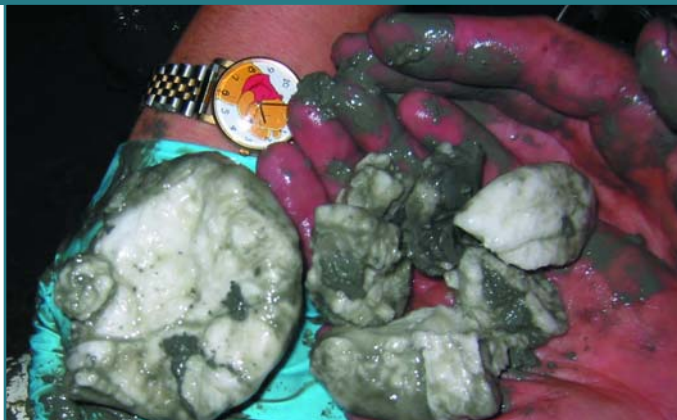
Chunks of gas hydrate recovered from a core taken in the Gulf of Mexico (USGS).
