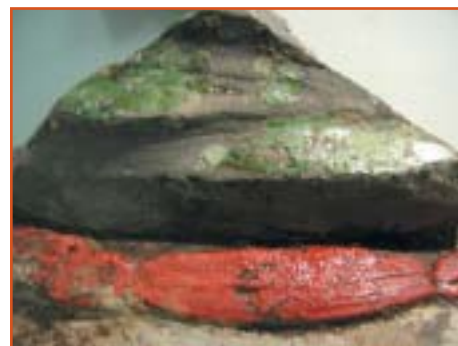
The shiny areas in this close-up of a terracotta fragment may appear wet, but they are actually solid HEMA that has polymerized at the surface. Photo courtesy of Heinz Langhals, Department of Organic and Macromolecular Chemistry, Ludwig-Maximilians University of Munich.
